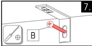
Caution! The wall must be examined before assembly. The included universal wall plugs are only suitable for use in firm masonry such as concrete block or brick. Do not use the wall plugs masonry such as hollow brick, lightweight block, surfaces such as gypsum plasterboard or other framing systems. If applicable, particular wall plugs must be used! These are available at a specialised store (hardware store). In case of non-compliance, the manufacturer/retailer or importer do not assume liability.
